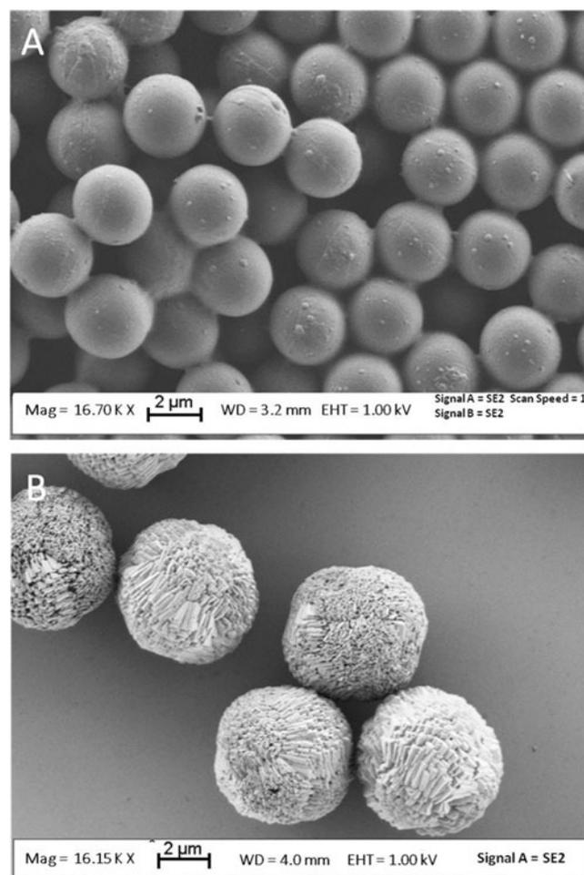
**Fig. 1** Scanning electron microscope (SEM) images showing **A** polystyrene spheres with 3  $\mu\text{m}$  diameter and **B**  $\text{MnCO}_3$  microparticles with 4  $\mu\text{m}$  diameter
